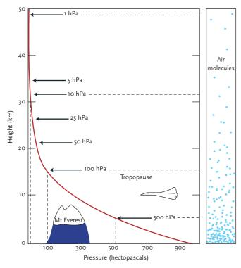
Figure 2-2 Pressure profile of the lower atmosphere at different altitudes
