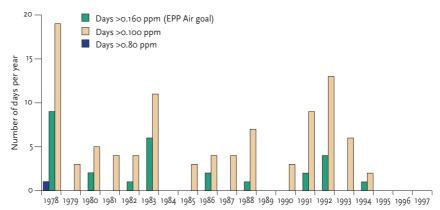
**Figure 2-45** Number of days during the year when the one-hour NO<sub>2</sub> concentration exceeded specified levels in south-east Queensland, 1978–97. Long-term levels are below the the EPP Air goal, tending to remain below 0.08 ppm.
