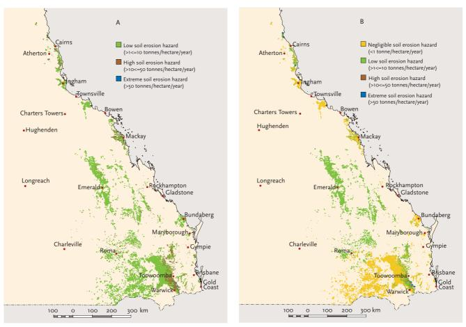
Figure 3-11 Water erosion hazard for broadacre crops and sugarcane under two management systems: A, stubble is incorporated and the land is left fallow, and B, stubble is retained and zero tillage is practised. (Source: DNR)
