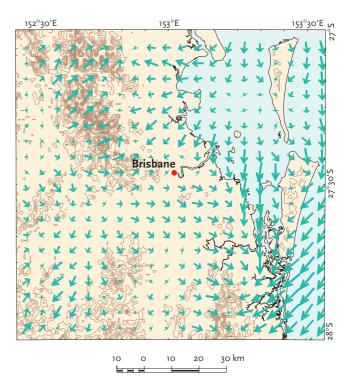
**Figure 2-57** Modelled winds and movement of pollutants emitted during the morning from around Brisbane on a summer day. The Lagrangian Atmospheric Dispersion Model (LADM), developed by CSIRO, predicts the detailed threedimensional winds, turbulent mixing and dispersion of pollutants in the course of a day.
