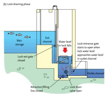
Figure 4-31 Walla Weir fish lock: stages of operation for downstream passage (Source: DNR)
