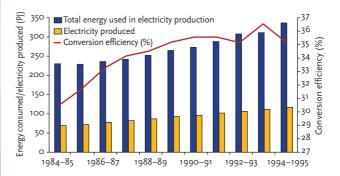
**Figure 6-11** Total energy used to produce electricity, electrical energy produced, and percentage conversion efficiency, 1984–85 to 1994–95 (Source: DME)
