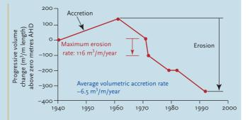
**Figure 5-10** Progressive sand volumetric changes on north Bribie Island, 1940–92. These data show a general trend of erosion (negative volume change) since 1961, with accretion (positive volume change) occurring only before that time.
