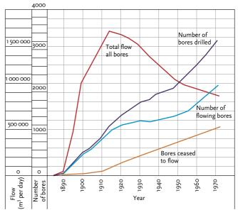
Figure 4-11 Number of bores drilled, flowing bores and nonflowing bores, and total flow to all artesian bores in Queensland (Source: AWRC 1975)
