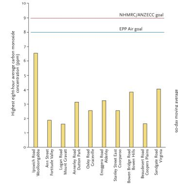
**Figure 2-55** Highest eight-hour average of carbon monoxide concentrations at ten Brisbane roadside sites, 1994–96. The NHMRC/ANZECC and EPP Air goals were not exceeded during the study.
