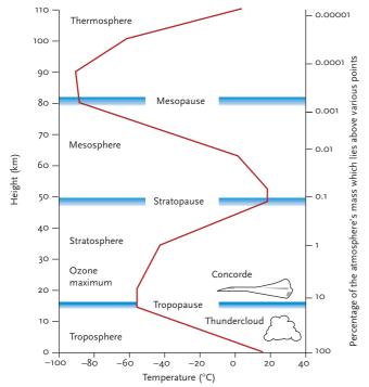
Figure 2-1 Temperature profile of the atmosphere at different altitudes
