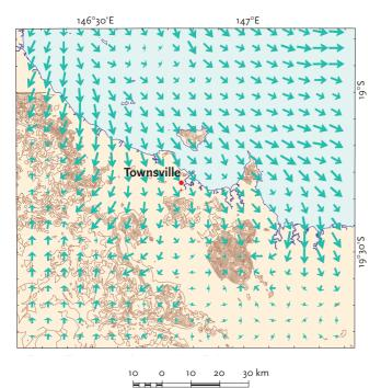
**Figure 2-59** Langrangian Atmospheric Dispersion Model of the Townsville area at 11 a.m. on a typical summer day, with the modelled sea breeze already moved inland 8 km to Mount
