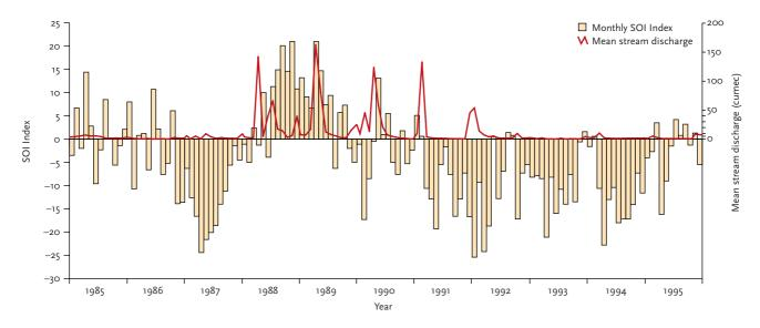
**Figure 5-14** Monthly discharge (m<sup>3</sup>/s) of the Logan River at Yarrahappini, south-east Queensland, 1970–96. The high variability in discharge and the influence of the El Niño drought between 1991 and 1995 are evident.
