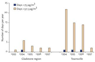
Figure 2-42 Number of days during the year when the 24-hour average  $PM_{10}$  concentrations exceeded specified levels in Gladstone, 1993–97, and Townsville, 1994–97 (no days above the EPP Air goal of 150 µg/m<sup>3</sup>)
