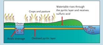
**Figure 5-3** Potential acid sulfate soils do not harm the environment when covered by water (a), but when drained and exposed to air — (b) and (c) — they react with rainwater to release sulfuric acid into the drainage system, affecting aquatic life.
